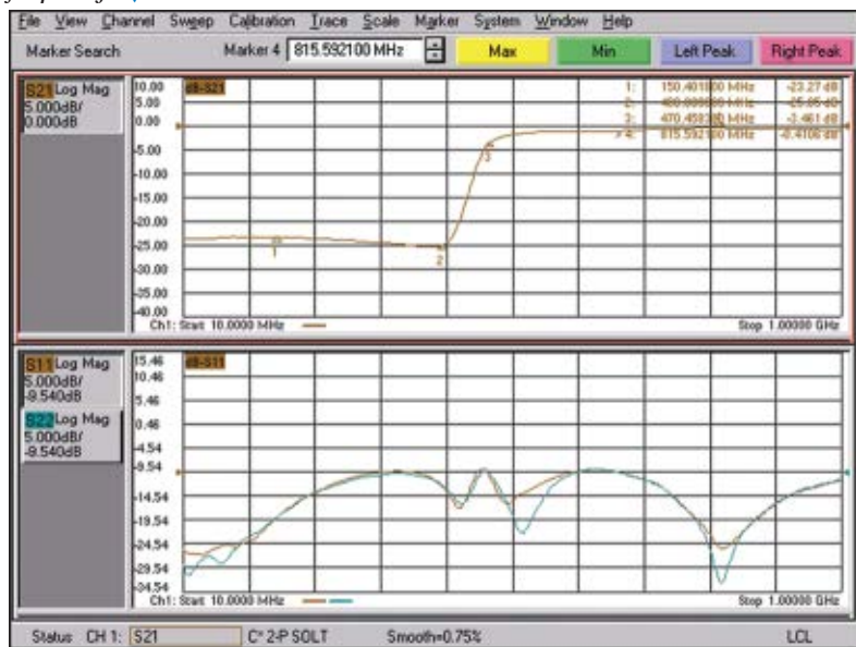
Fig. 1 The limited rejection high pass filter's insertion loss and return loss vs. frequency. ▼
